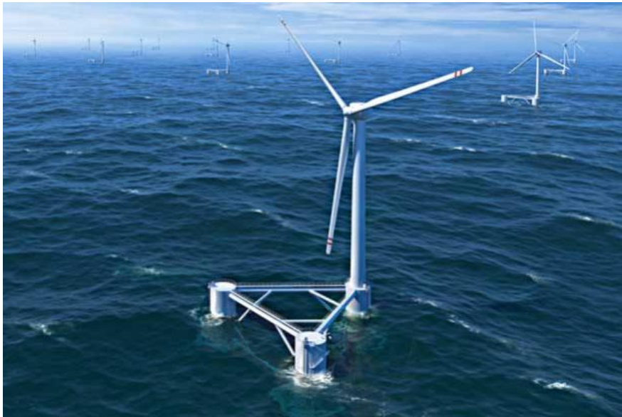
Principle Power says the stability of its foundation means that it can be sited in deep water, out of view from the shore Photograph: Principle Power
